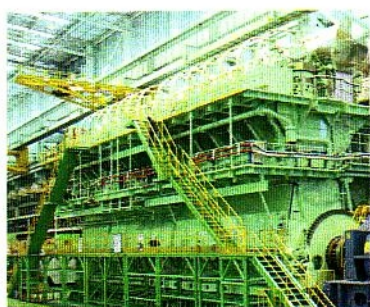
Wärtsilä Engine Type RT-flex96C-B, max. 80'800kW @ 102rpm
