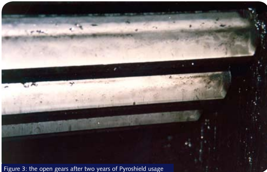
Figure 3: the open gears after two years of Pyroshield usage
