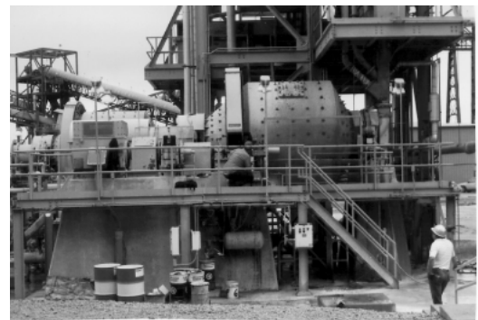
Koppers Ball Mill Unit A
