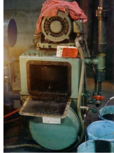
Stokes vacuum pump model 212-11 with access with access cover removed. Note the plate is covered with carbon prior to converting to LE's 8420 MONOLEC GFS Engine Oil.
