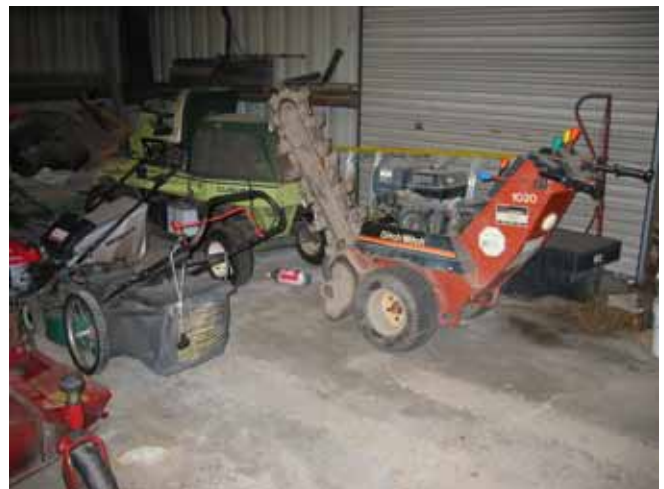
Lawn mowers, Cushman diesel mowers and 1020 Ditch Witch trencher
