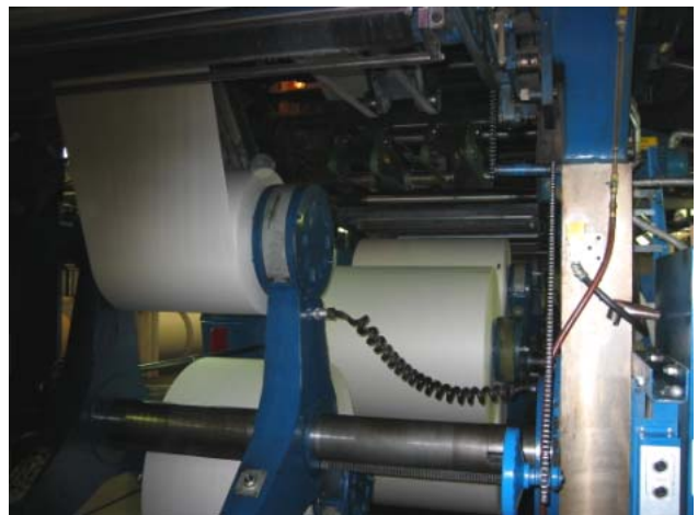
CT50 Reel Tension Paster – handles 50 inch dia. rolls
