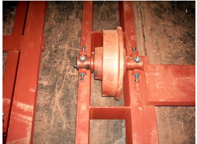
Kiln car wheels during assembly (above and below)
