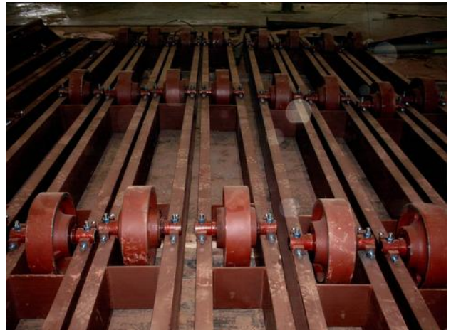
Kiln car wheels during assembly (above and below)
